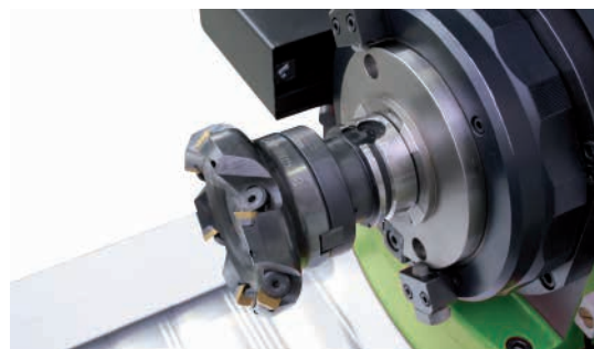
Modular precision spindles for the highest degree of reproducibility when changing different insert modules.
