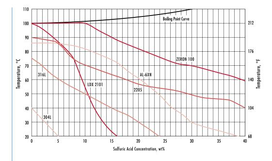
Sulfuric Acid Iso-corrosion Curves, 4 mpy Stainless Steels
