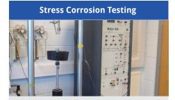
Slow strain rate testing rig, 2L & 5L autoclave corrosion testing.
